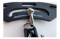
\* Mast rake can be measured by measuring the angle difference between transom and mast. This needs to be done with 140kg shroud tension and can be done with your phone by using a level app
