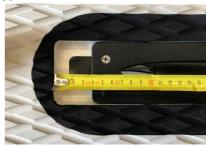
\* Clew position Jib is the position of the shackle on the clew board.
