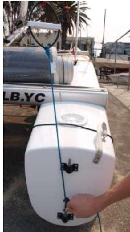
The standard setting, for 150kg crew weights is the top screw on the plastic rudder clip.
