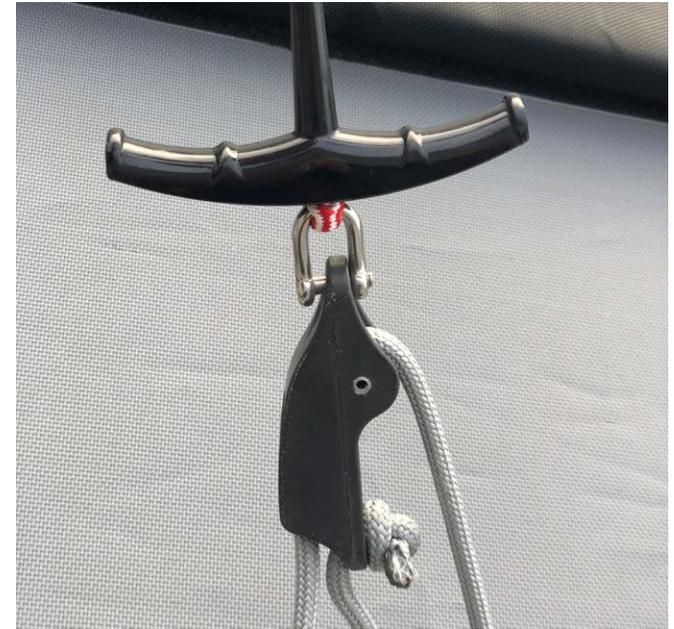
7. Knot the adjustable trapeze line to the trapeze shockcords.
