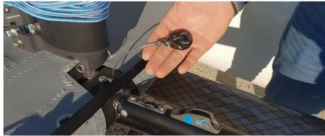
2. Feed the spinnaker halyard first through the 29mm T2 block and then through the 40mm block located on the mast.
