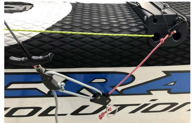
**Check if the shrouds and trapeze lines are in the right order before raising the mast!**
